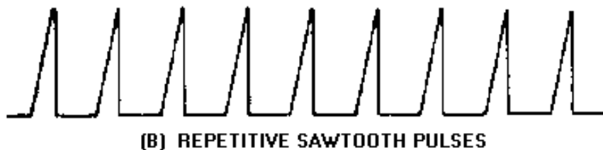
Figure 2-44B.—Pulse-duration modulation (pdm). REPETITIVE SAWTOOTH PULSES.
