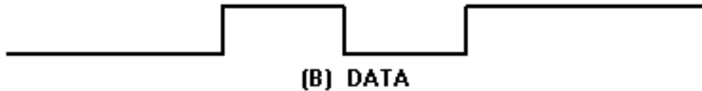
Figure 2-26B.—Simulated phase-shift keying. DATA.
