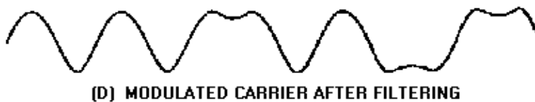
Figure 2-25D.—Phase-shift keying. MODULATED CARRIER AFTER FILTERING.
