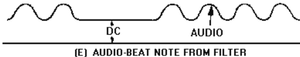
Figure 3-3E.—Heterodyne detection. AUDIO-BEAT NOTE FROM FILTER.
