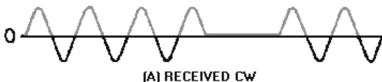
Figure 3-1A.—Cw demodulation. RECEIVED CW.
