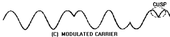
Figure 2-25C.—Phase-shift keying. MODULATED CARRIER.
