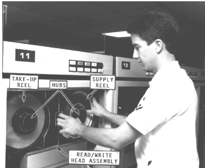
Figure 2-12.—Mounting a magnetic tape
